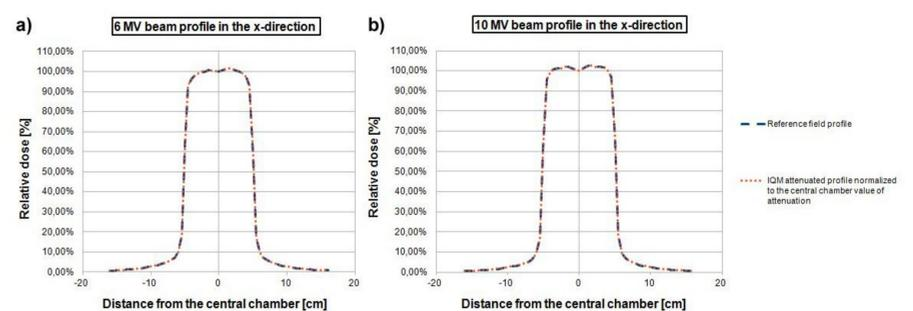
Figure 2. Beam profiles in the X directions for a 10x10 cm<sup>2</sup> field for: a) 6 MV photon beam; b) 10 MV photon beam. The reference field profile (blue line) is plotted with the IQM attenuated field normalized to the average attenuation value (orange line).
