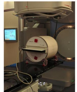
Figure 1. Experimental setup: linac-head integral quality monitor (IQM) and RT-smartIMRT phantom
