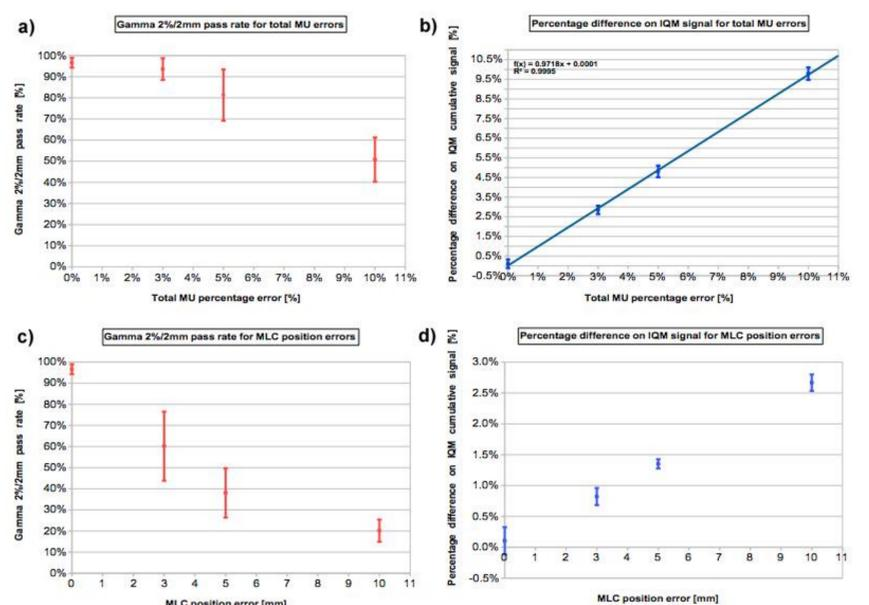
Figure 3. Results for VMAT plans: a) Gamma pass rates for MUs variations; b) IQM signal percentage differences for MUs variations; c) Gamma pass rates for MLCs shift; d) IQM signal percentage differences for MLCs shift.
