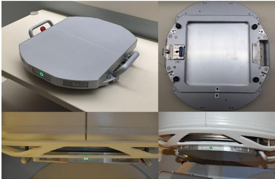
**FIG. 1.** The Integral Quality Monitor (IQM) is a large area ion chamber (top left) with a gradient of the ion chamber thickness in the axis of MLC motion. It attaches to the accessory tray holder, similar to an electron cone (top right). The device has a low profile from the linac head (bottom left and right) and connects wirelessly to a transceiver and the controlling computer.
