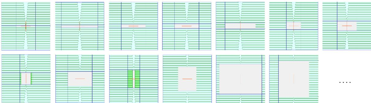
**Figure 1** Example apertures which are commonly employed to empirically determine an array of Area Output Factors (AOF). The AOF is a basic requirement for the machine-specific commissioning of the IQM calculation algorithm.
