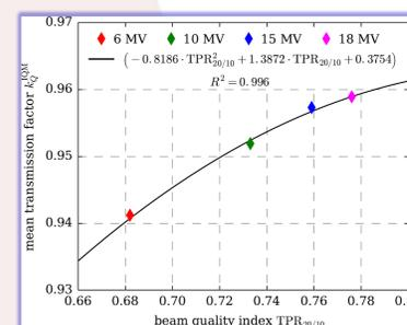
**Figure 4.** Mean transmission factors  $k_Q^{IQM}$  of IQM versus beam qualities TPR<sub>20,10</sub> for investigated set of standard flattened beams. For every investigated beam energy and radiation field size, data represent average values of measurements from all participating institutions.
