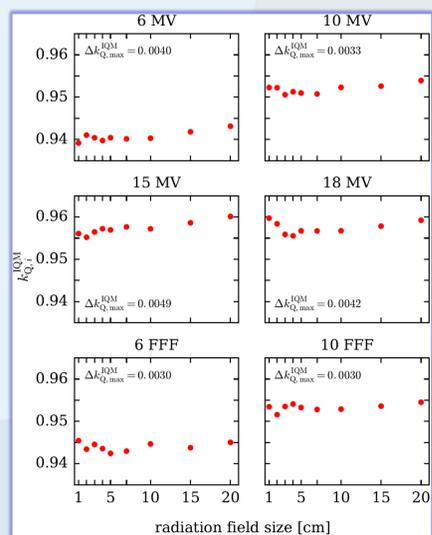
Figure 3. Transmission factors  $k_{Q,i}^{IQM}$  of IQM versus radiation field size, for each nominal beam energy. Data represent average values of measurements from all participating institutions.  $\Delta k_{Q,i}^{IQM}$  denotes maximal difference of  $k_{Q,i}^{IQM}$  for a given nominal energy.
