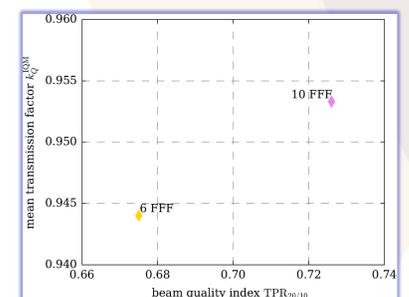
**Figure 5.** Mean transmission factor  $k_Q^{IQM}$  of IQM versus beam quality TPR<sub>20,10</sub>, aggregated by nominal energies 6 MV FFF and 10 MV FFF photon beams.
