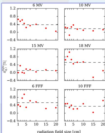
Figure 1. Changes in beam quality  $\delta_{Q,i}^{IQM}$  versus radiation field size for investigated beam energies when IQM was mounted on the linear accelerator. For every beam energy and radiation field size, data represent average values of measurements from all participating institutions. Dashed lines represent mean differences  $\delta_Q^{IQM}$  for a given energy.
