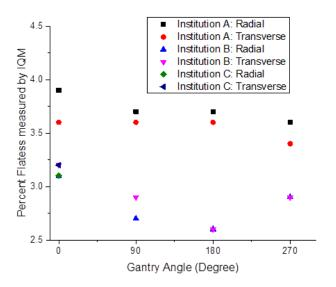
The **beam symmetry constancy**, for both the radial and transverse directions, for all cardinal gantry angles, are found to be **within 0.5%** for institution A. while for institution B the consistency was **within 1%**.
