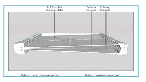
Large area ionization chamber with a gradient in the electrode plate separation (in the axis of MLC motion)
