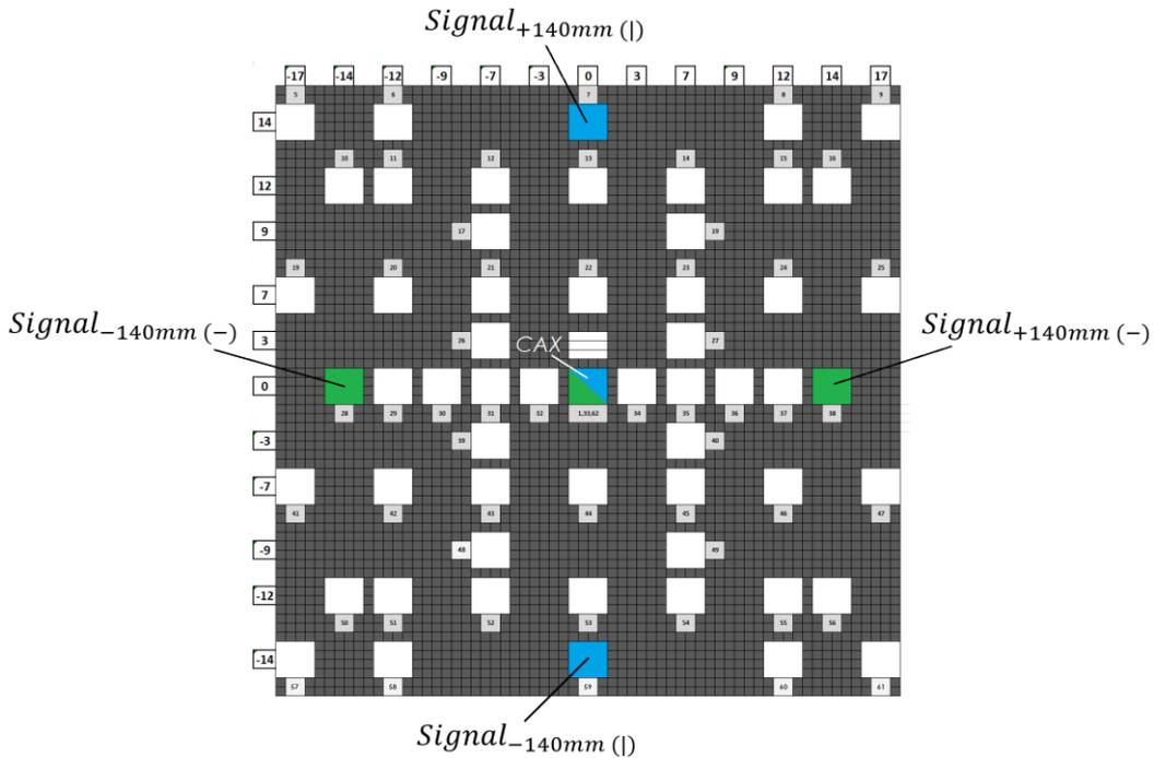
**Figure 2** Geometry of the 4x4 cm<sup>2</sup> apertures of the IQM QA-plan, commonly used for IQM model validation and machine QA. The plan is intended to scan the whole 40x40 cm<sup>2</sup> beam profile covered by the active detection area of the IQM chamber. The highlighted segment's signals were used to calculate symmetry and flatness values.
