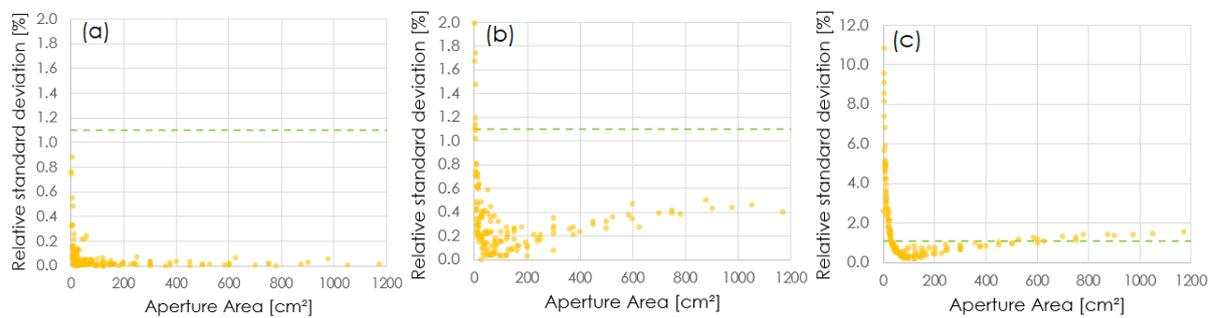
**Figure 3** Standard deviations ( $SD_{AOF}$ ) between IQM signals for a set of rectangular fields (AOF) relative to the referring average signal, measured at: (a) the same Linac with the same detector on the same day, (b) two matched Linacs with different chambers, (c) nine unmatched Linacs with different detectors. The single-machine single-session tolerance of 1.1% for  $SD_{AOF}$  is represented by the green, dashed line.
